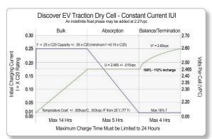
NOTE: This algorithm uses a pulse termination criterion. As a safety precaution during the Finish phase, if the average cell voltage, or volts per cell (vpc), exceeds V2 and the charger output has been on for more than 30 seconds, the output is shut off until the vpc falls to V3. The finish phase then resumes and this "pulsing" continues until the target overcharge (108% - 112%) is reached.
